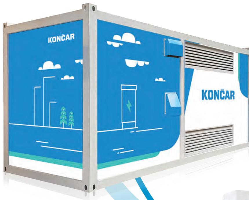
**The *KonCharge 1000* battery charger is a power converter specifically designed for charging batteries onboard rail vehicles, including both full battery and hybrid powertrain systems. It operates with an input voltage of 10(20) kV and is capable of parallel charging two batteries, each with a power rating of up to 500 kW.**
