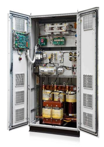
The rectifier can be configured with an optional diode-based dropper unit, enabling simultaneous supply of loads at nominal voltage and charging of batteries at a higher boost voltage, thereby optimizing charging cycles.
