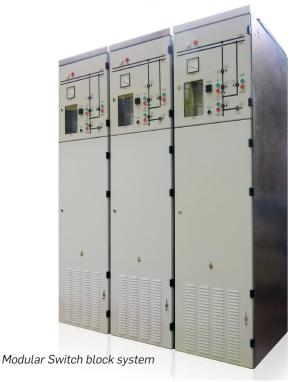
The upper section, located behind the front door, houses the control, monitoring, and protection systems, including protective MCB breakers for 48 V DC and 24 V DC auxiliary power supplies, signal terminal blocks, a USZMR relay for feeder field protection and control, and a central PLC controller for automation and system management.
