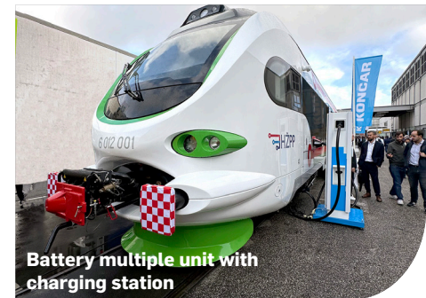
Battery multiple unit with charging station
