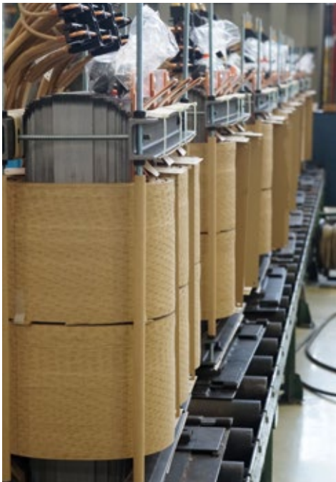
Manufacture of distribution transformers
