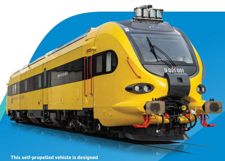
This self-propelled vehicle is designed to monitor, measure, and record track conditions with precision. Built on the reliable platform of our current electric and diesel-electric trains, this high-floor vehicle is powered by a diesel engine and can reach speeds of up to 140 km/h on both electrified and non-electrified tracks.
