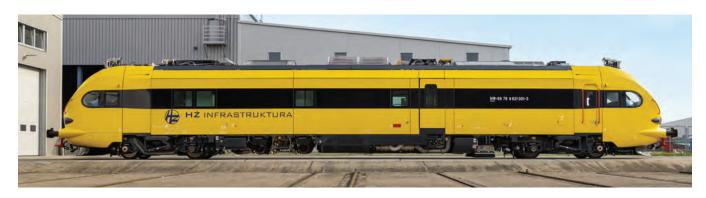
It features a track gauge of 1435 mm and measures 25 meters in length, 2885 mm in width, and 4280 mm in height, with a floor height of 1250 mm above the track.
