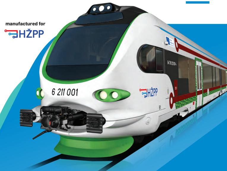
Battery Electric Multiple Units (BEMUs) leverage a 25 kV, 50 Hz AC traction system for propulsion and battery charging, reaching speeds of 120 km/h in battery mode and 160 km/h when connected to the overhead line. They accommodate up to 300 passengers.
