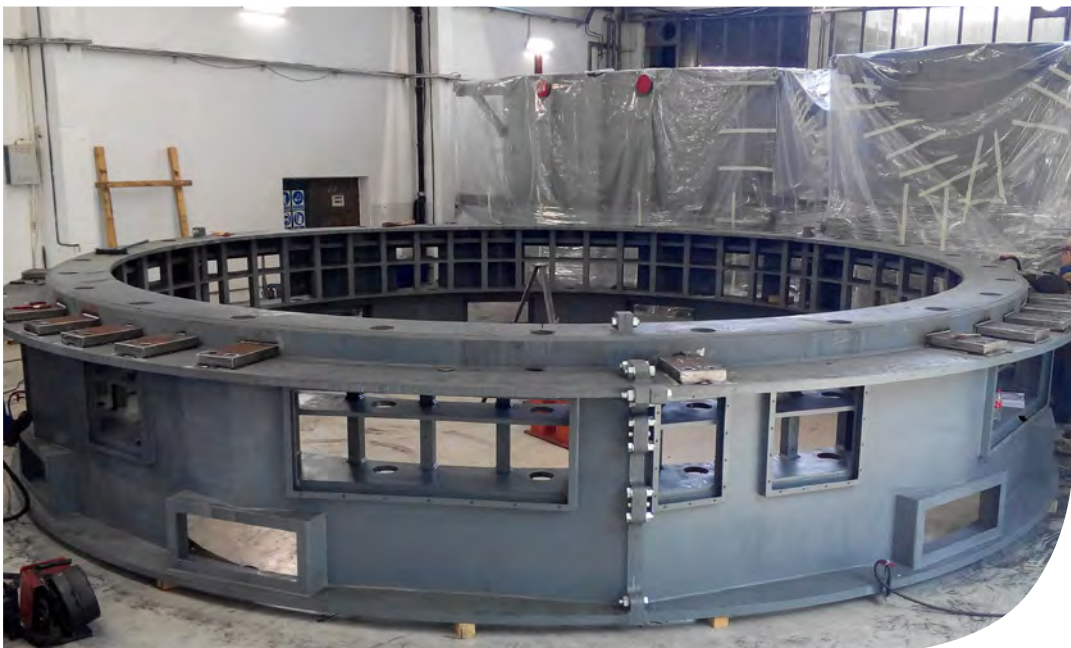
Hydro-generator – stator frame
