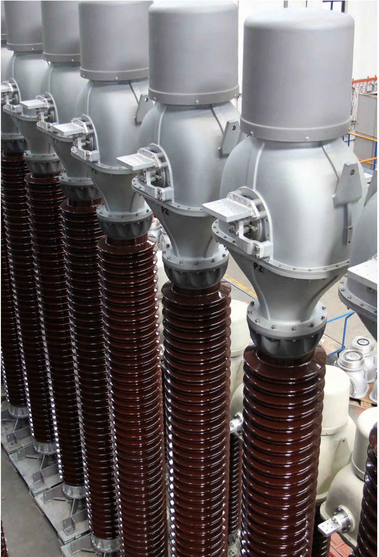
Current transformers 525 kV delivered to Russia
